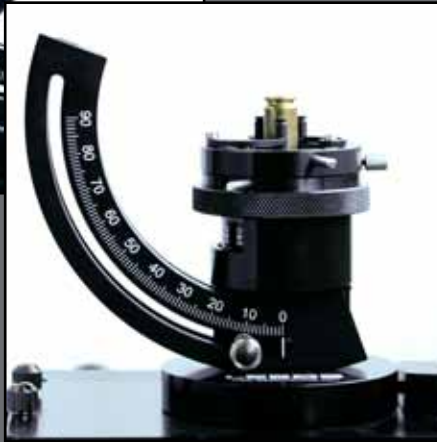
.40-caliber casing held by the exterior
