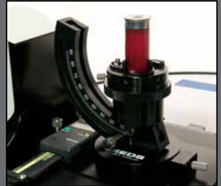
12-gauge shotgun shell held by the outside diameter
