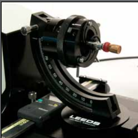
Bullet mounted to a pin mount with sticky wax
