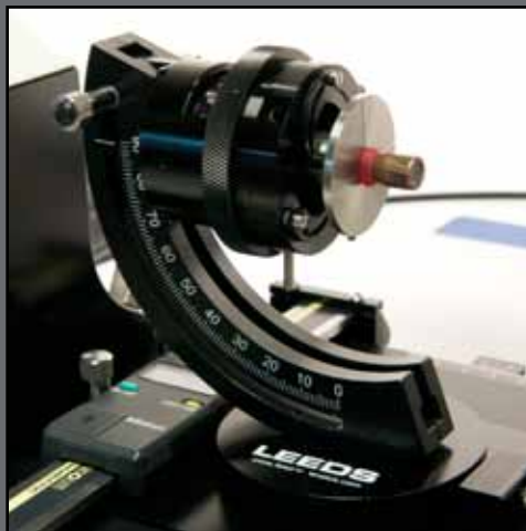
Bullet mounted to a mini-platter with sticky wax
