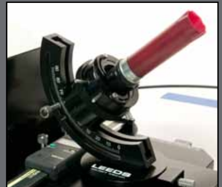
12-gauge shotgun shell held with the Leeds Magnetic Shell Mount
