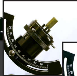
.40-caliber casing held by the extraction groove
