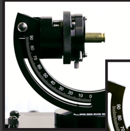
.40-caliber casing held by the inside diameter
