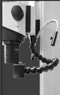
CROSS BAR MOUNT flexible tube arm, column mount
