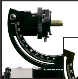
.40-cartridge casing held by the inside diameter
