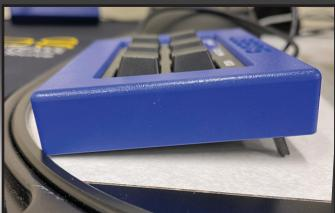
*Leeds Six- Button Key Pad* is a tactile controller for the Leeds LCF3 or Discovery Comparison Microscopes to control the table height, column height, and fluroscent light controls.
