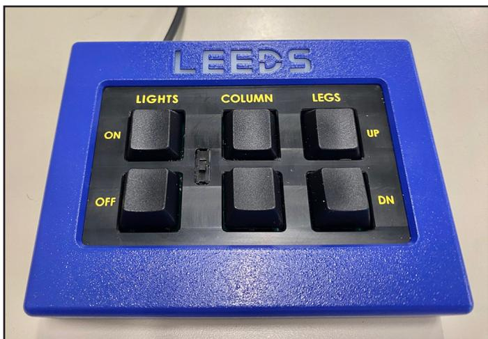
**Leeds Six-Button Key Pad** is a tactile controller for the Leeds LCF3 or Discovery Comparison Microscopes to **control the table height, column height, and fluorescent light controls.**
