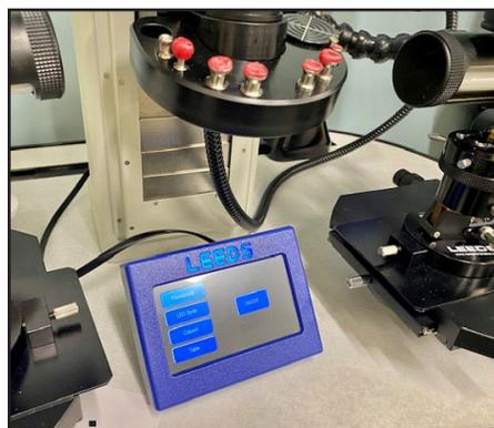
The new tactile Six-Button Controller is an alternative to the touchpad on your Leeds LCF3 or Discovery microscope
