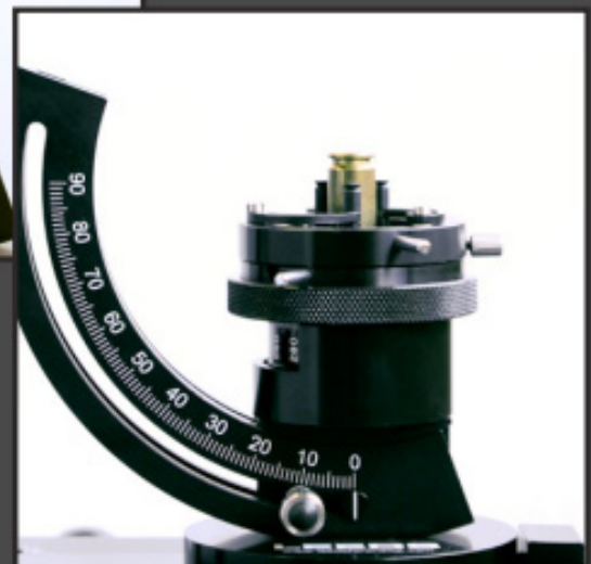
.40-cartridge casing held by the outside diameter
