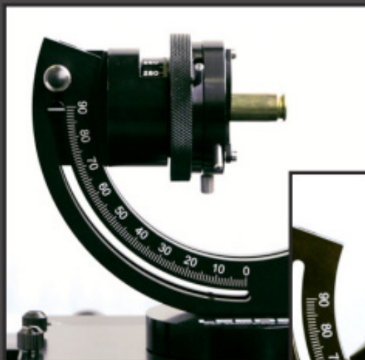
.40-cartridge casing held by the inside diameter
