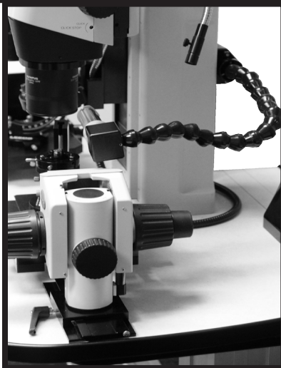
Gooseneck arm mounted on back of column
