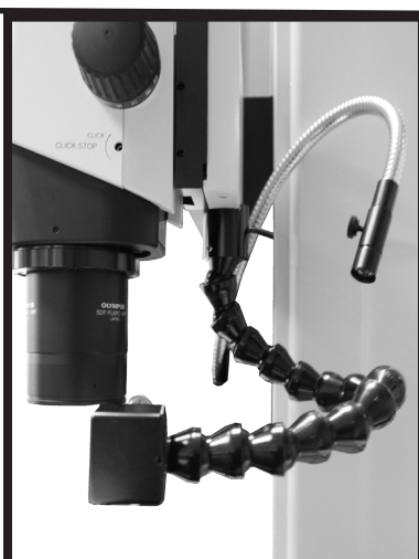
Gooseneck arm mounted on front of column
