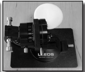
LCF-BDWT Contrast Disc provides a white backdrop to a bullet or cartridge case when loaded in the Leeds Universal Holder and viewed through a Leeds comparison microscope. The Contrast Disc is secured with a screw and can be swiveled in and out of viewing range as needed.
