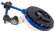
Light Guide Positioner: Used to record and duplicate the distance from sample, height, angle of illumination, and rotary position. Useful for reverse lighting technique.
