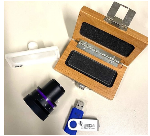
Leeds Calibration Kit: 200 division stage micrometer; reticle with 200 divisions; slide holder; flash drive with instructions & templates
