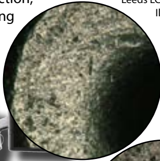
Breach face viewed through Leeds LCF3 with Fluorescent Illumination
