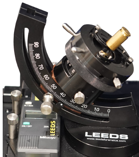
.40-caltridge casing held by the extraction groove
