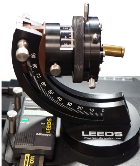
.40-caltridge casing held by the inside diameter
