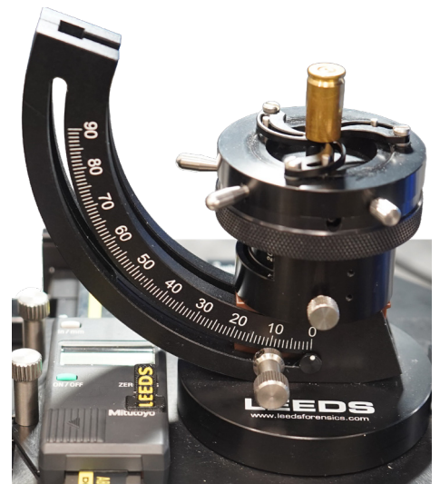
.40-caltridge casing held by the outside diameter
